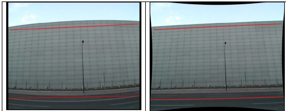
Figure 2: Calibration for image perspective and distortion
