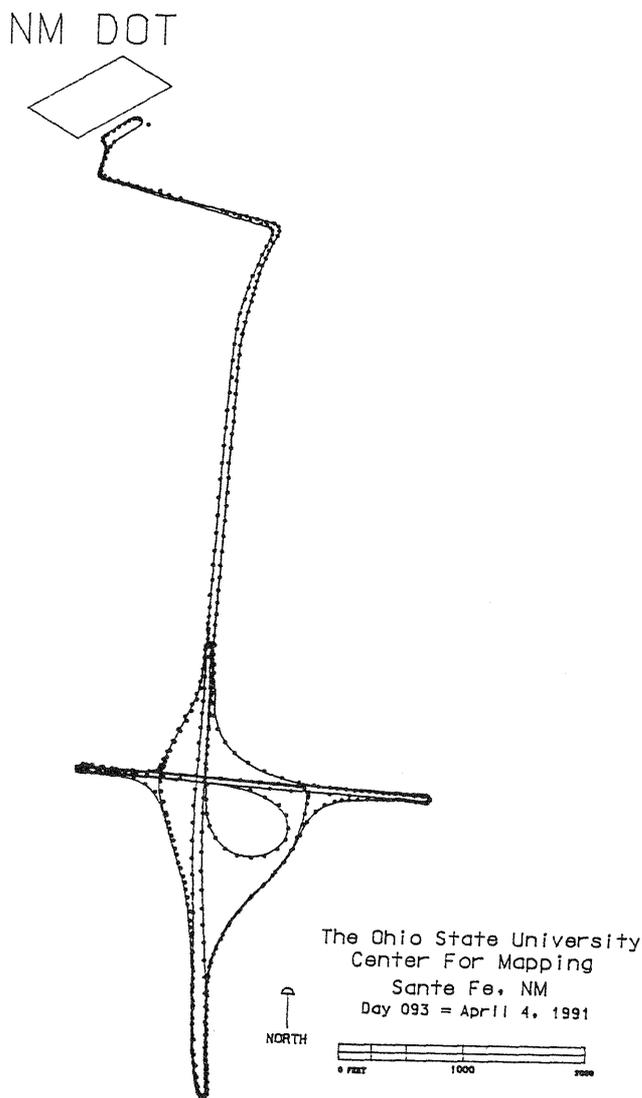
Figure 2: Resulting alignment of a combination of inertial and GPS observations. The circles indicate position fixes by GPS.
