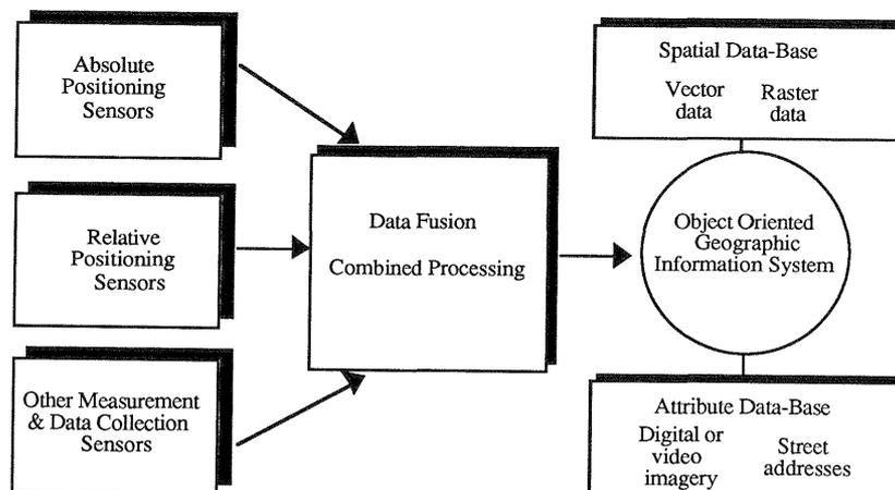
Figure 1: Conceptual design of a mobile mapping platform that integrates various sensors, data-analysis functions, and an object oriented data-base.
