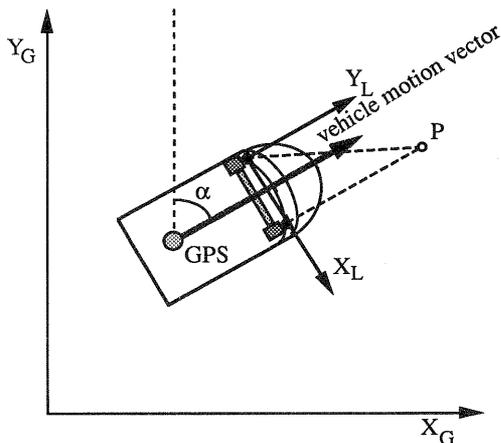
Figure 4: Transformation of relative positions determined with the stereo-vision system into the absolute coordinate frame.
