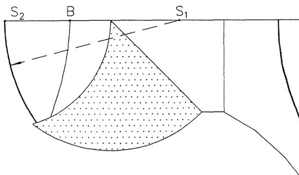
Figure 4: Lines and area (cone of revolution) of equal slope on the surfaces as defined in Figure 1.
