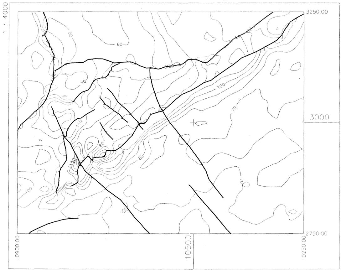
Figure 7: Lines of equal terrain slope, interval 10 %
