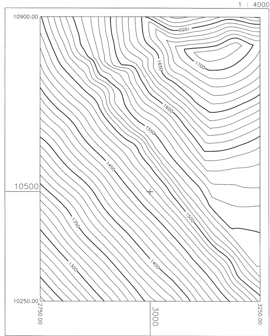
Figure 5: Contour lines with interval 10 m.
