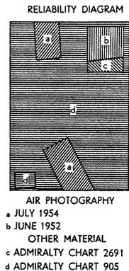
Figure 5 - Typical example of a reliability diagram which may be found on a topographic map. The visual variable orientation has been used to show the various data sources (Fiji 1:50 000, DOS, 1964).
