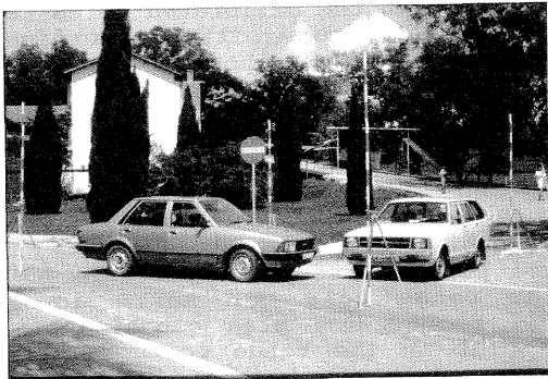
Fig. 4. A photograph of a simulated accident site taken with a non-metric 35- to 70-mm zoom camera, showing "preferred" range pole arrangement.
