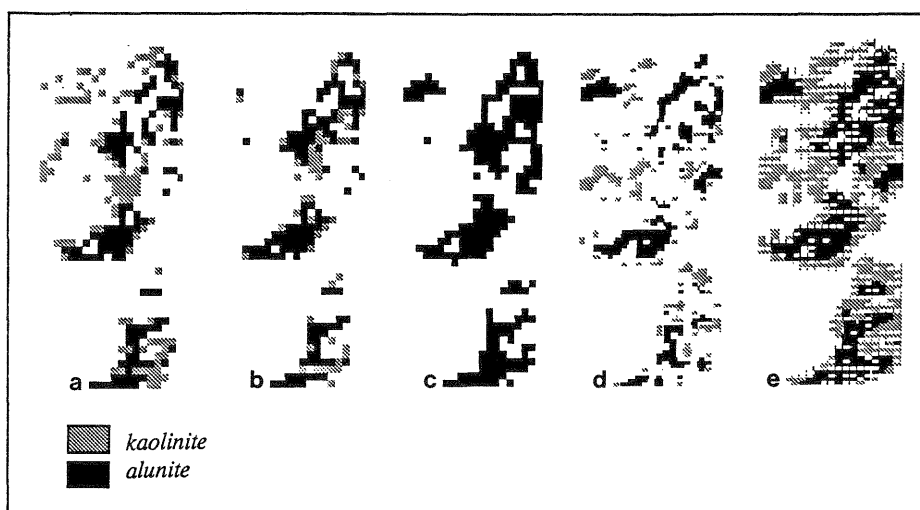
Figure 4: Classification results for ground classes Kaolinite and Alunite using (A) Box classification, (B) K-Nearest neighbour analysis, (C) maximum likelihood decision rules, (D) indicator kriging using probability values greater than 0.5, and (E) indicator kriging using probability values greater than 0.
