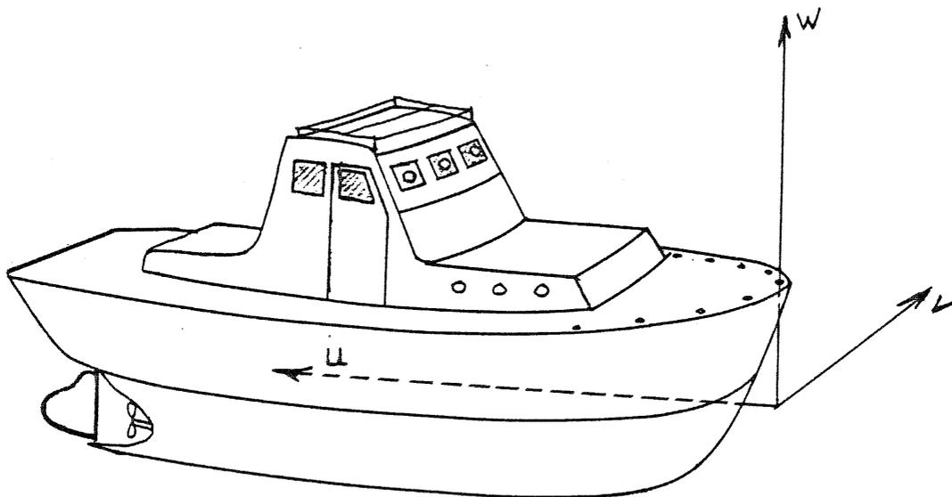
Fig. 1. The boat's coordinate system.
