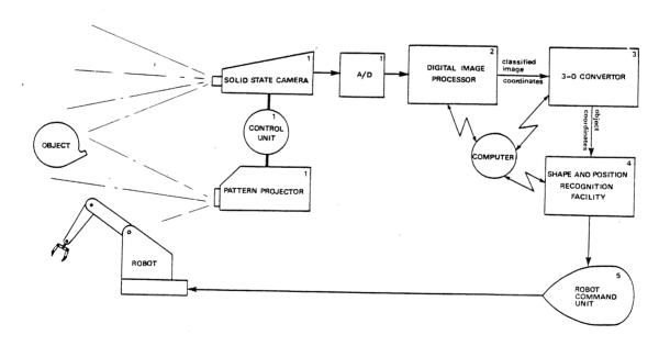
FIGURE 1: Elements of the Robot-Vision System
