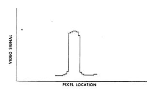
FIGURE 5: Video Signal at and Near Projected Line
