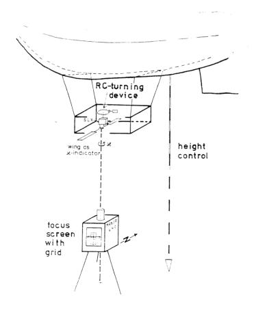
The accuracy with which the airship could be positioned by this method worked out at 1-2m in its position, the angle of swing could be kept down to 5 gon.
