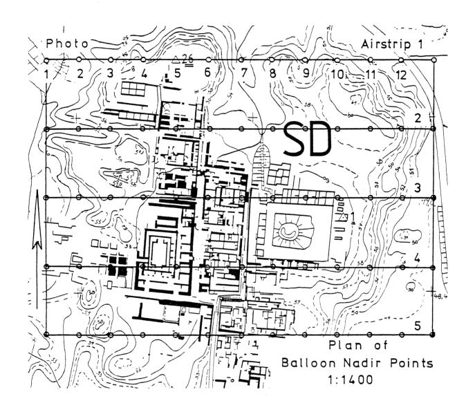
For the exposure a Mamiya 645 reflex camera was set up on a tripod over each BNP, aligned, with the optical axis in strict vertical, and orientated on a N-S axis by means of a compass. A cross-hair focusing screen was used as viewfinder.
