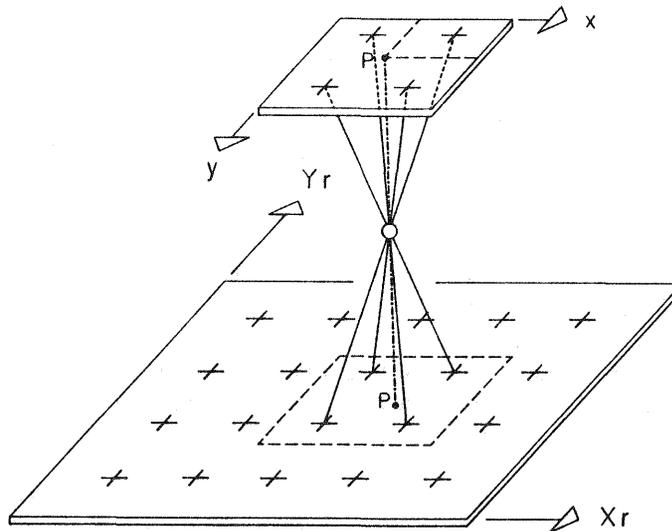
Fig. 1: The principle of reseau-scanning
