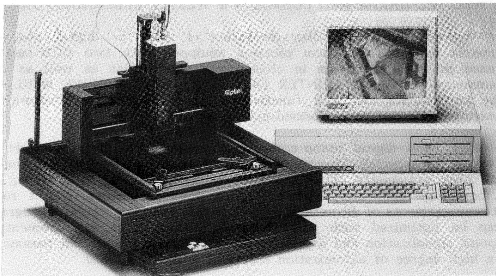
Fig. 2: Digital mono-comparator Rolleimetric RS1
