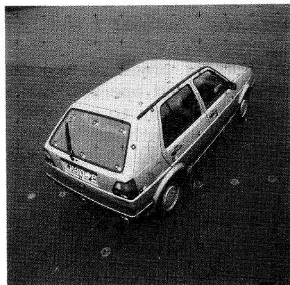
Fig. 7: a) test field triangulation
