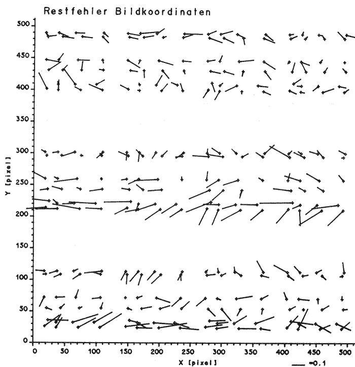
Fig. 3: Sensor distortion (residuals of image points)
