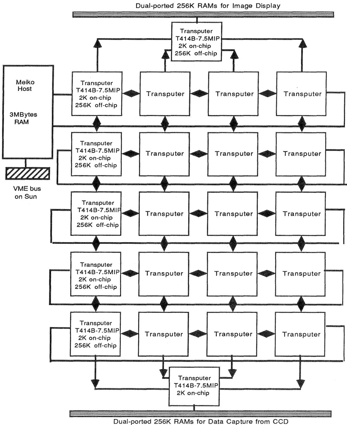
Figure 3 : Schematic diagram of Meiko transputer array at RSRE Malvern
