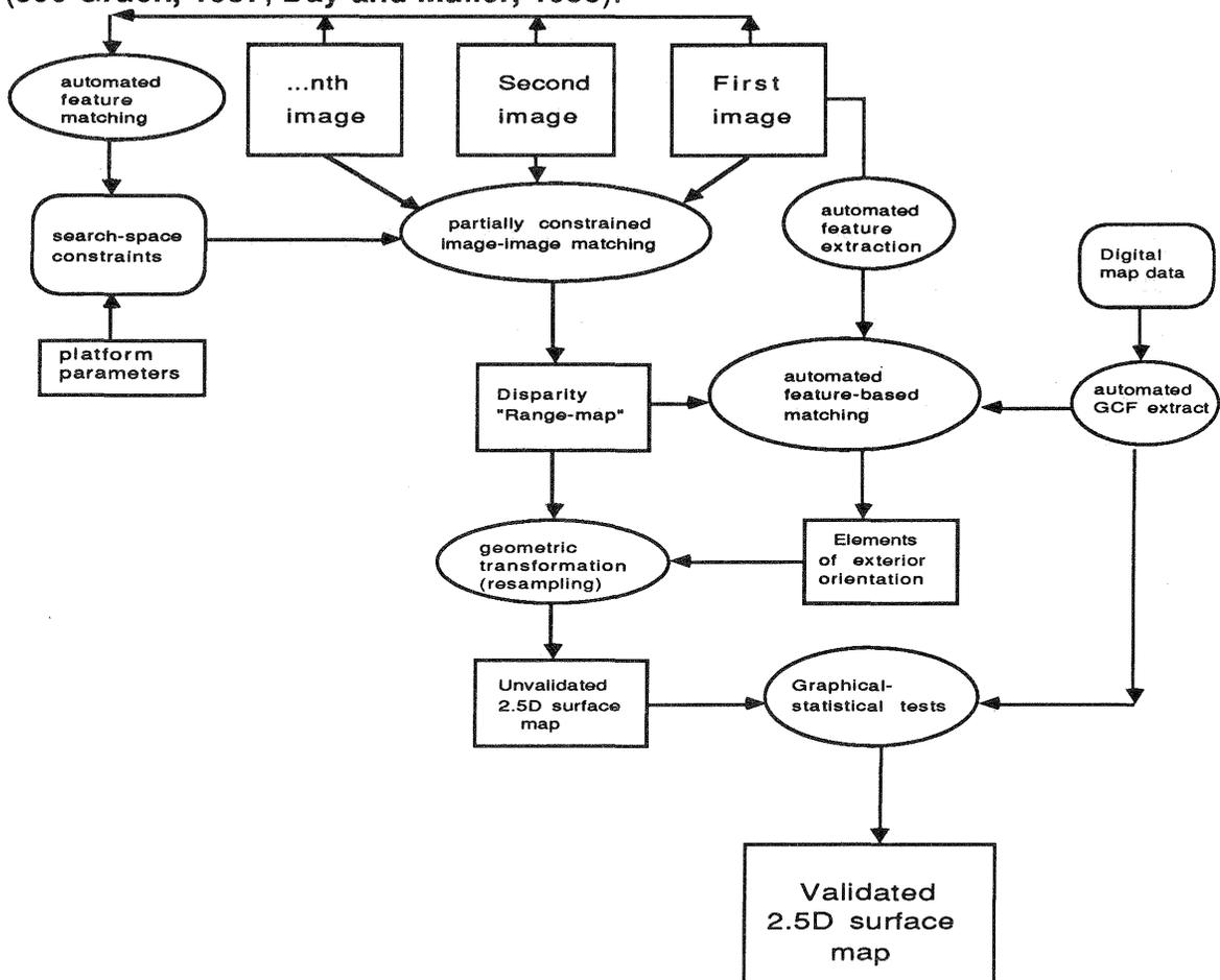
Figure 1 : Schematic diagram of system components for automated SPOT stereo matching
