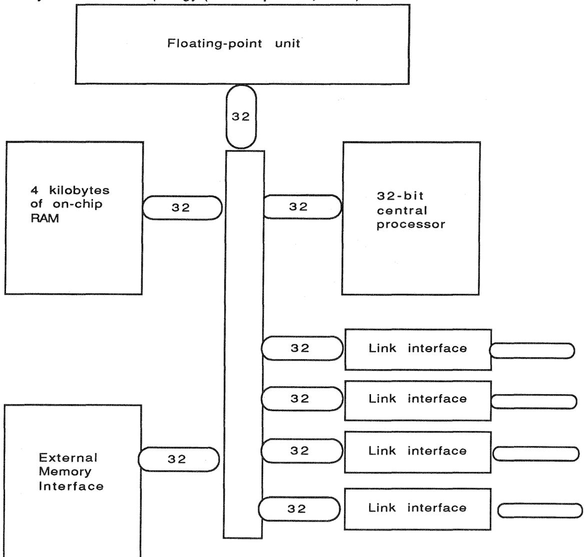
Figure 2 : Schematic architecture of T800 floating-point transputer
