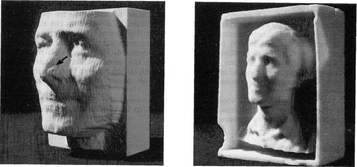
Fig. 4. N.C. milled surfaces of a face.
