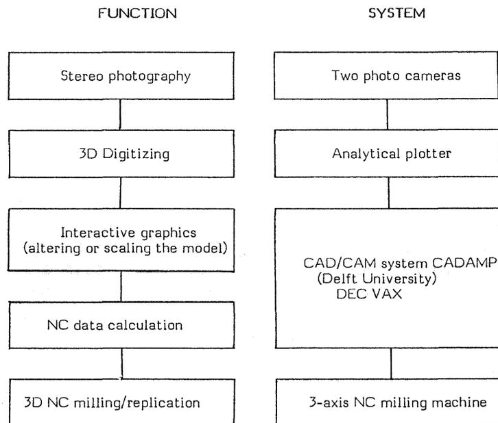
Fig. 1. Overview of the production system and the apparatus and software used.
