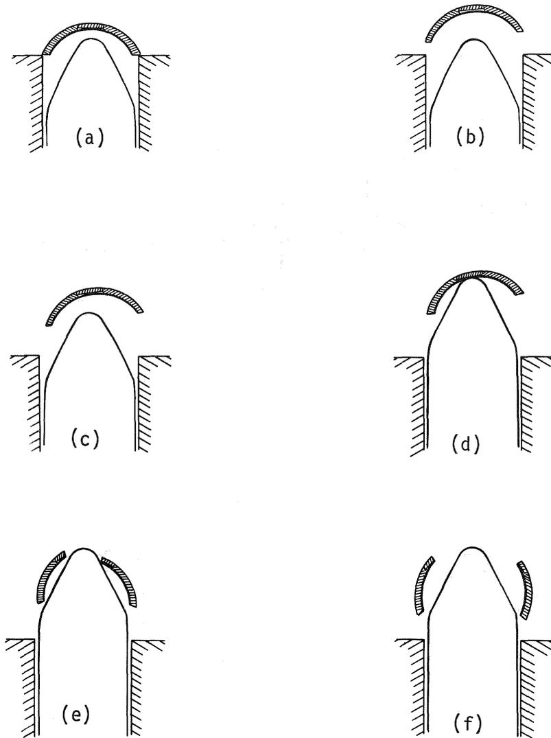
Figure 3: Interaction of TV and closure during a test event
