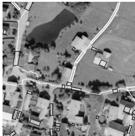
Figure 7: Detail: Global link hypotheses (dotted, white) and road segments (start segments for global grouping are white, others, black).
