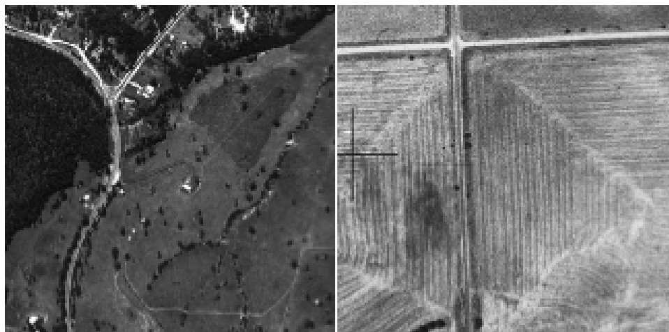
Figure 2: The images used for testing the 2D transform domain least squares matching algorithm. The “Redland” image (left) was formed by taking a square region of size 1600 \times 1600 pixels and subsampling using a 10 \times 10 Gaussian window. A stereo pair with a known uniform disparity of 0.5 pixels was created by introducing a 5 pixel horizontal displacement, then subsampling as before. The “Willunga” image (right) was formed by taking a square region of size 328 \times 328 pixels and subsampling using a 2 \times 2 Gaussian window. A stereo pair with known uniform disparity of 0.5 pixels was created by first displacing the image by 1 pixel, then subsampling.
