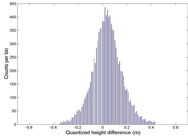
Figure 4: Histogram of the relative height discrepancy between the 1<sup>st</sup> strip and the 2<sup>nd</sup> strip.
