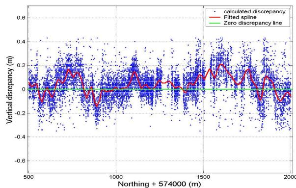
Figure 5: Relative height discrepancy in North-South direction (overlap region between the 1<sup>st</sup> and the 2<sup>nd</sup> strip).
