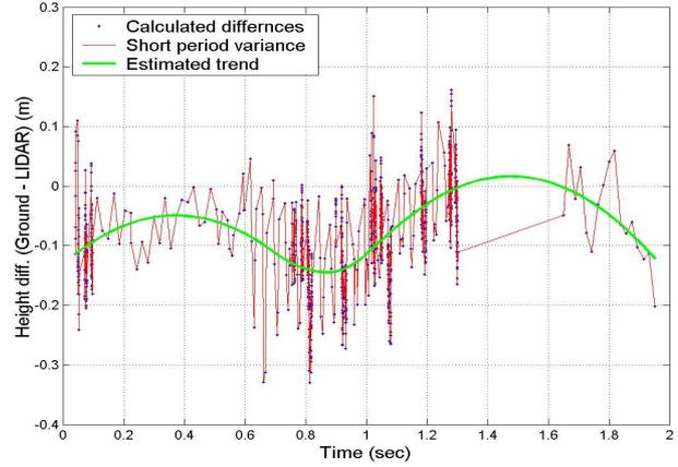
Figure 9: Height accuracy (Ground - LIDAR) versus time.
