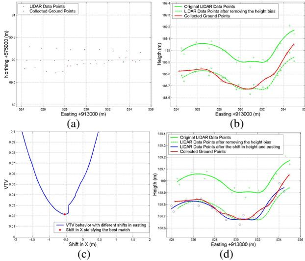
Figure 8: Planimetric offset in (X) direction at location EW3R.
