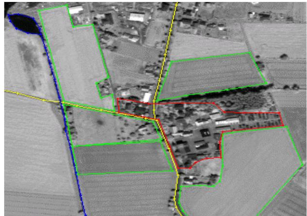
Figure 4 Linear network and area features in an orthophoto derived from an aerial image. Features (blue for water, green for fields, red for settlement, yellow for roads) have been derived semi-automatically.
