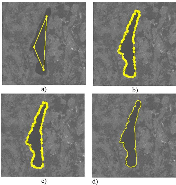
Figure 3 2D-parcel extraction for a lake feature in an IKONOS scene. a) Start position by operator. b) Result after first run. c) slight improvement after 2<sup>nd</sup> run. d) Final result with strong generalization.
