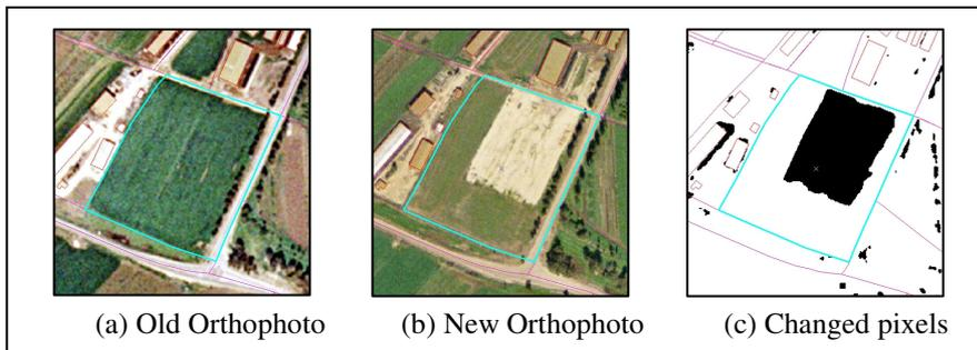
Figure 4: Example of changed pixel cluster which was detected as a part of large area object.
