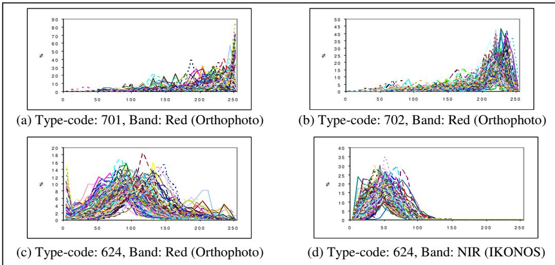
Figure 2: Examples of grey level distributions on pixels within unchanged objects sorted by object types and spectral bands.
