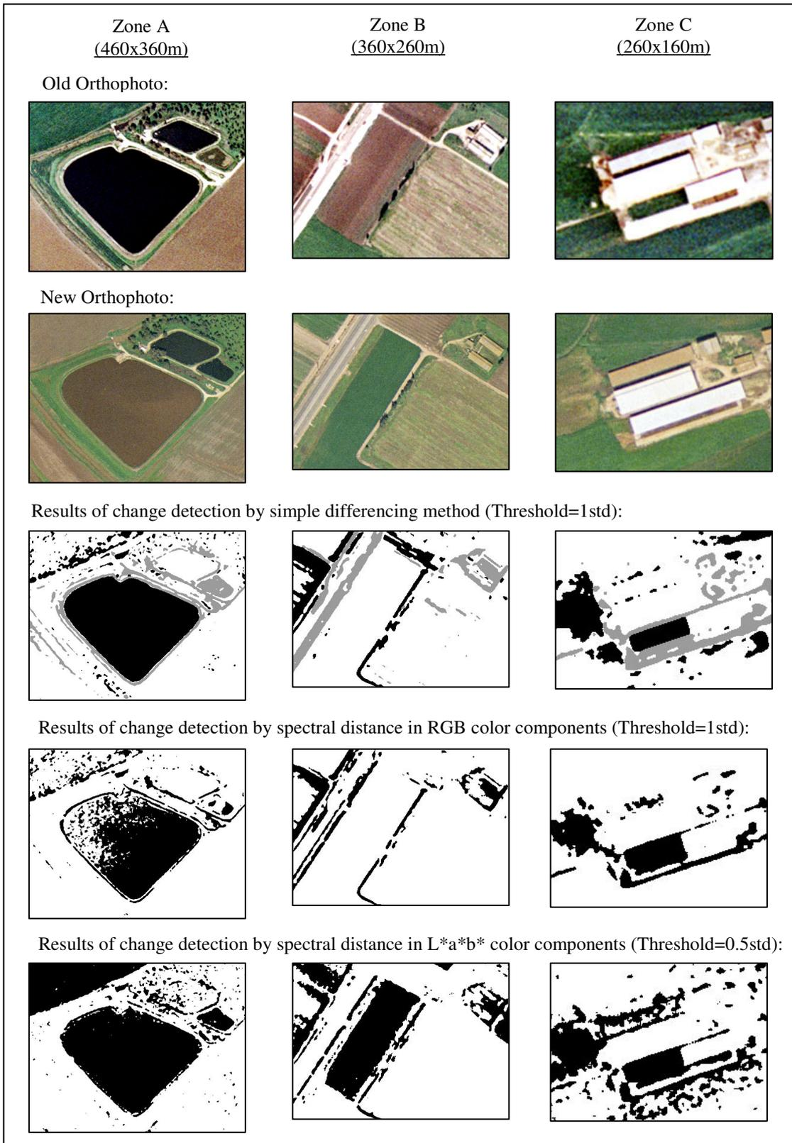
Figure 1: Examples of results of change detection experiences in three different zones and using three methods. Shown are the enhanced results by 5x5 majority filter.
