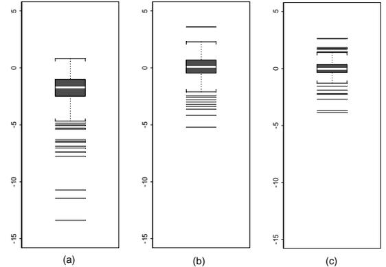
Figure 3: Box plots of the discrepancies of leveling measurements with (a) original D-InSAR measurements, (b) error-detrended measurements, and (c) integrated measurements.
