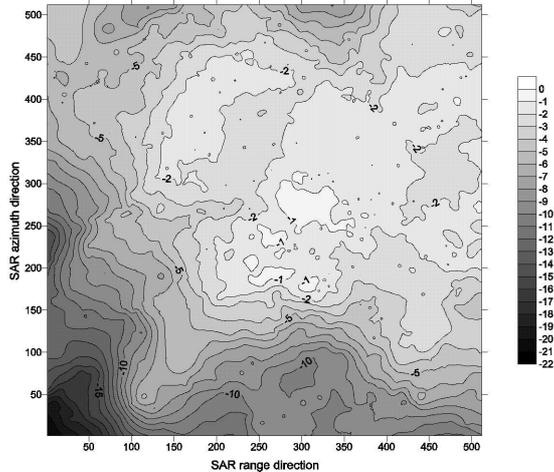
Figure 2: Contour map generated from the calibrated D-InSAR height change measurements (cm). Coordinates are expressed in pixels with a size of 40 by 40 m.
