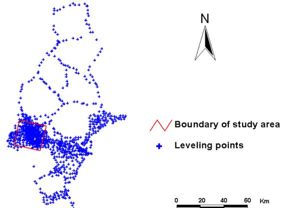
Figure 1: The leveling network established in Tianjin to monitor land subsidence. The total length of the leveling routes equals 3,000 km. The study area is indicated by a rectangular boundary.
