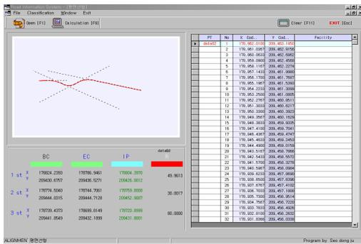
Fig. 13. Horizontal alignment information system
