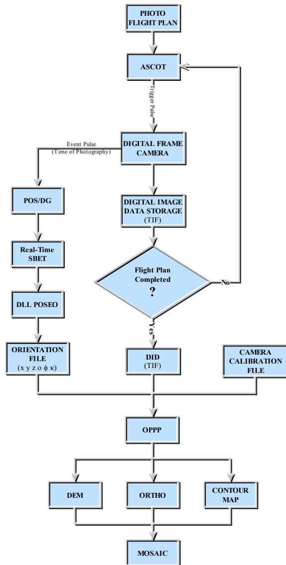
Figure 3. RTPMS general processing flow.
