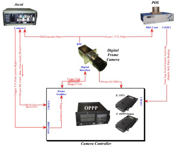
Figure 4. Hardware integration of the OPPP with the DFC, POS, and ASCOT.
