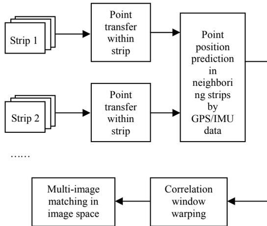
Fig.1 Workflow of point transfer method
