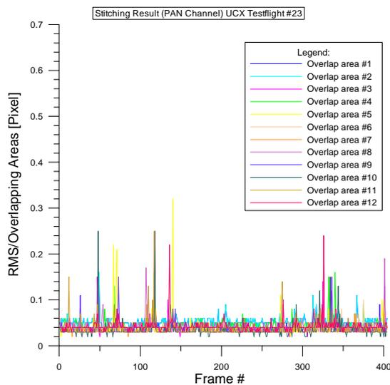
Fig 2: RMS error of matched stitching points
