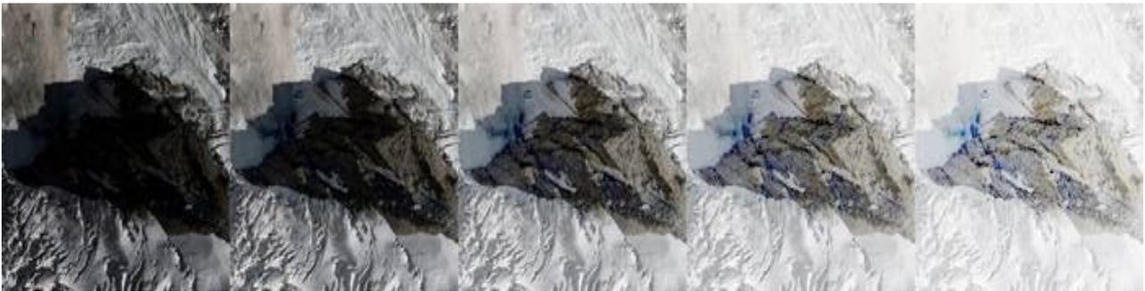
Fig. 7: Aerial image of very high intra scene contrast (snow and ice vs. shadows and dark rocks). Different gamma settings were applied to show details of different brightness.
