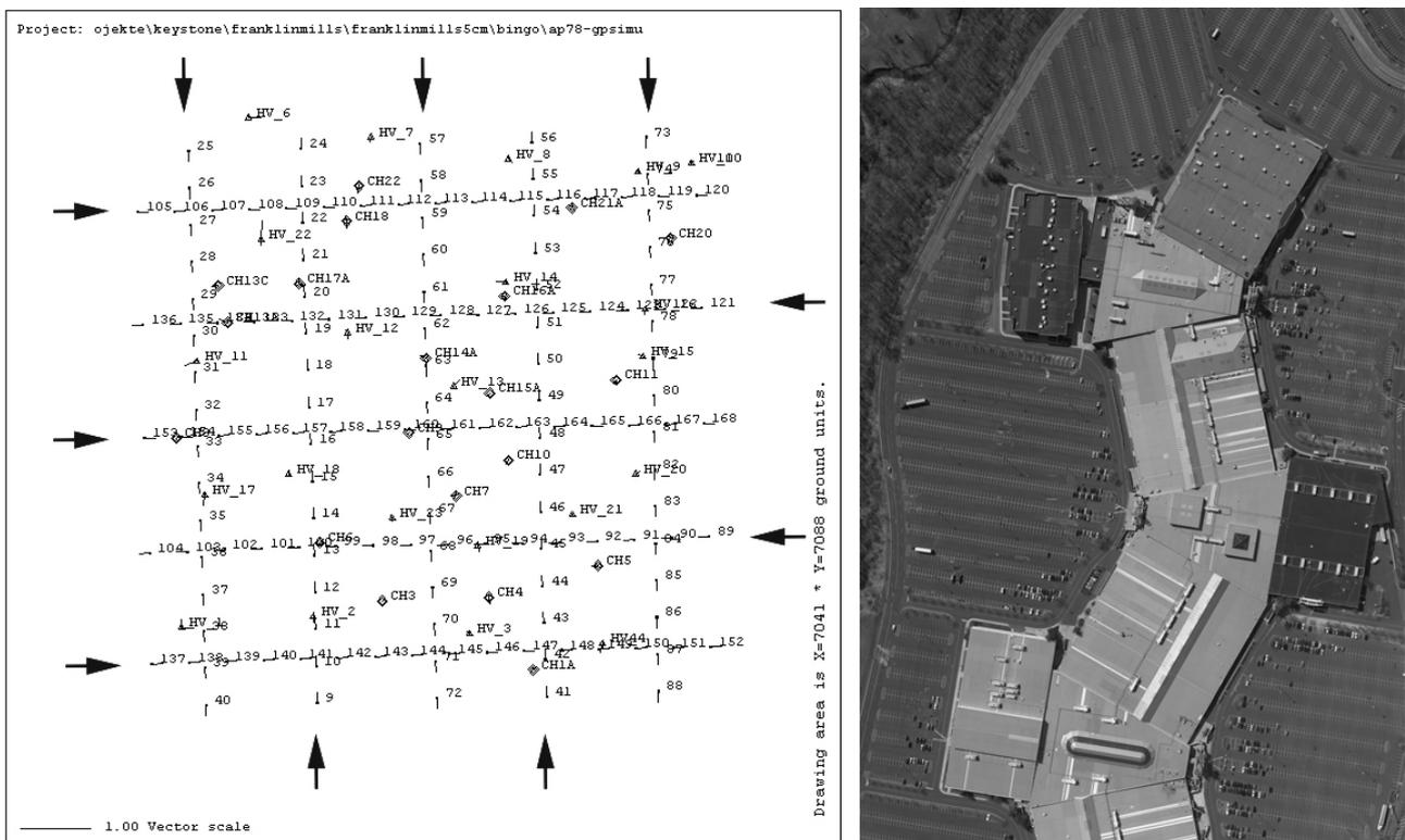
Fig. 8: Test area Franklin Mills near Philadelphia. The flight plan shows 10 flight lines with 160 images at high overlap (80% / 60%). The cross track pattern enables to carefully analyze the geometric property of the images. On the right: Frame 93 of the flight mission on March 25<sup>th</sup> 2008 performed by Keystone Aerial Surveys, Philadelphia, VA.
