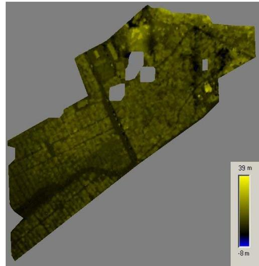
Figure 8. Difference DSM between 2000 and 1975
