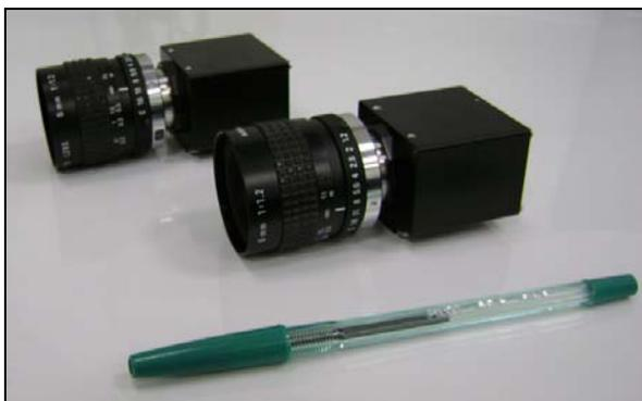
Figure 6: Prosilica GC1020 cameras
