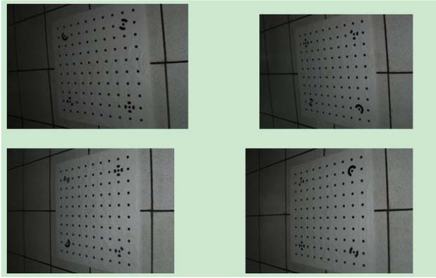
Fig.3 The third four images of the model plane. They are photographed with the camera rotated 90 degrees clockwise.
