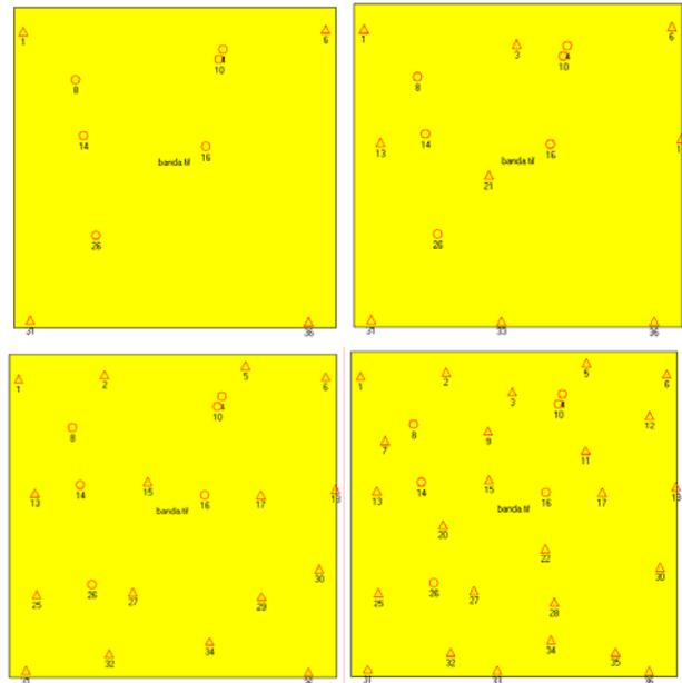
Figure 3. The GCP and Check Point distribution in each 4 sets (GCPs = triangles).
