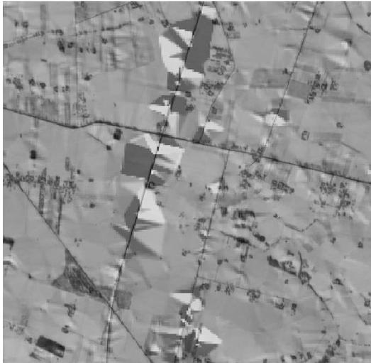
Figure 3. Gross errors identification using Blend Tool in ERDAS Imagine
