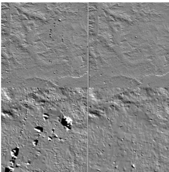
Figure 4. DSMs calculated in LPS 9.0 (left) and LPS 9.2 SP1.
