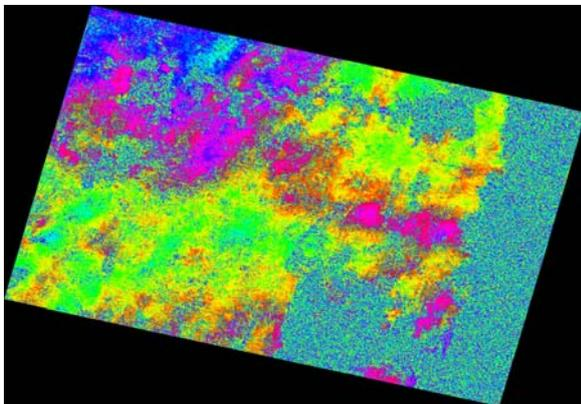
Figure 6. Interferogram of test site using DInSAR
