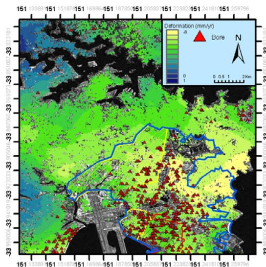
Figure 8. Deformation result using PSInSAR
