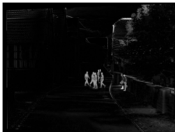
Figure 5: Temporal difference between a reference view with a view transformed by a homography.
