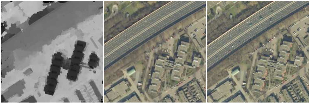
Figure 6: Expected value of depth (left) and the estimated orthoimage y^* (middle). One of the input images is shown right. Note that the cars disappear in the estimated ortho image.
