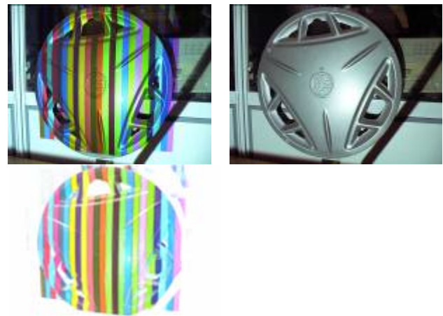
Figure4b: Industrial part right images. Same as Fig 4a, from top left: Slit pattern projected image. White light image and subtracted image.
