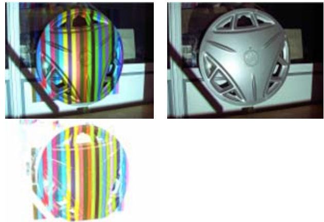
Figure4a: Industrial part left images. From top left: Slit pattern projected image. White light image and subtracted
