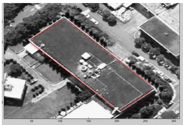
Figure 11. Projection of extracted lines on the aerial image
