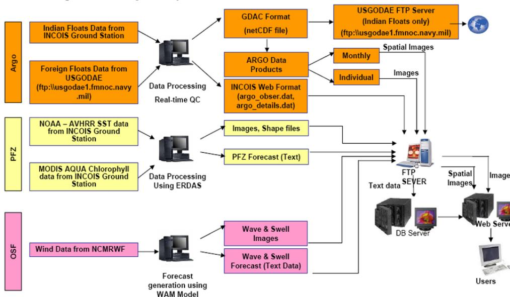
Figure 3. Flowchart describing the data reception, processing and web-services
