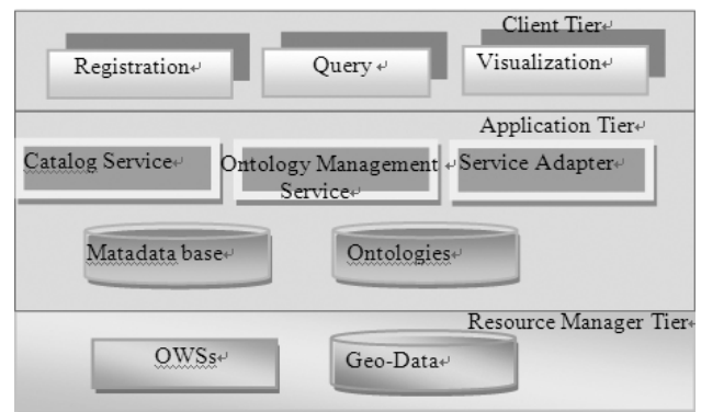
Figure 2. Architecture for integration of GI service
