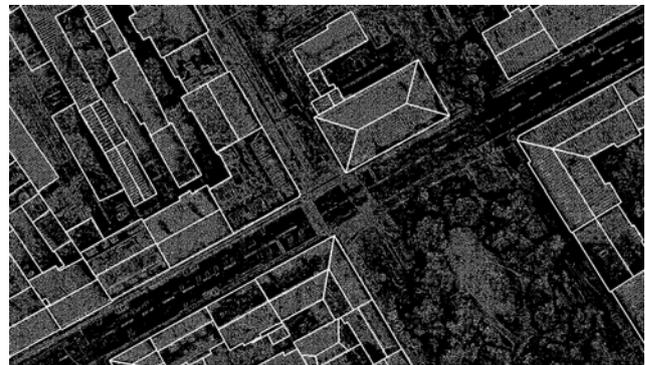
Figure 3. Extracted building from MATCH-T DSM point cloud
