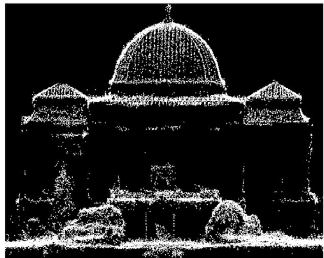
Figure 1. True 3D filtered MATCH-T DSM point cloud from aerial images
