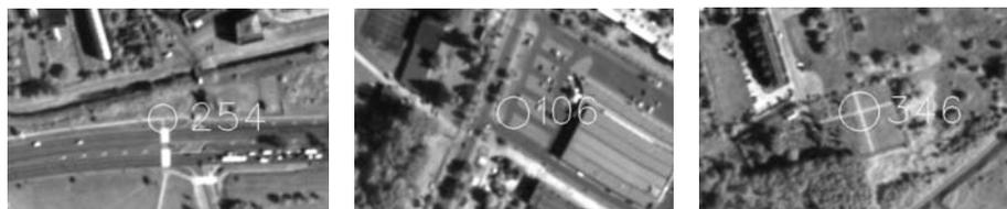
Figure 1. The project of ground control points on the Resurs DK-1 images
