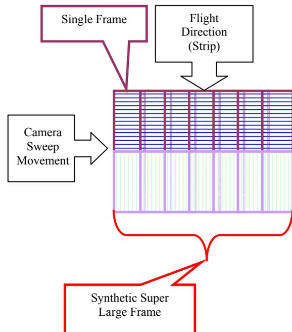
Figure 2. Flights with the VisionMap A3 Camera
