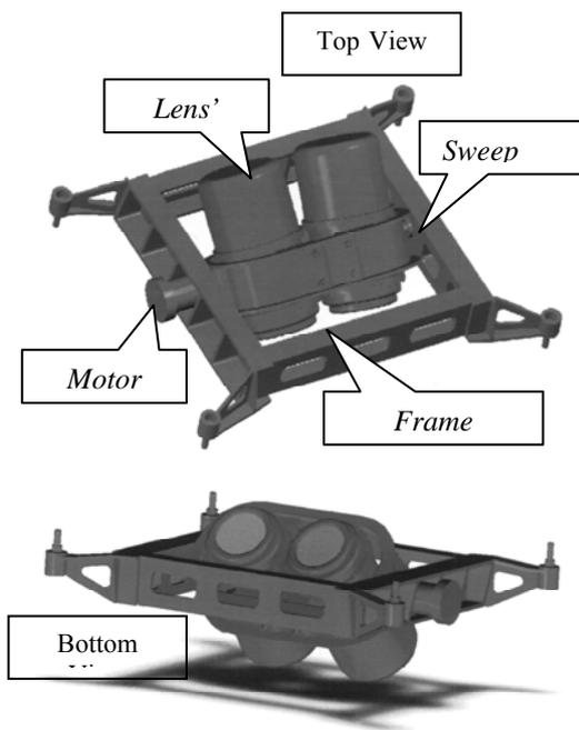
Figure 1. Camera Module Design
