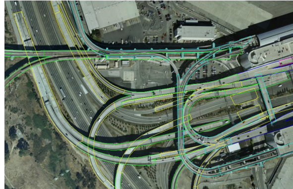
Figure 8, Even if no correction of building lean in the orthoimage is required, elevated freeway structures must be dealt with
