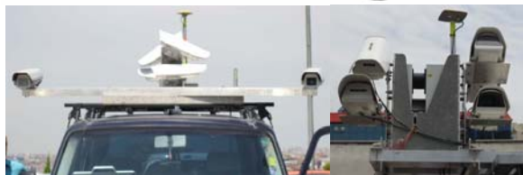
Figure 4. Sensor configuration on the mobile mapping van of VISIMIND AB
