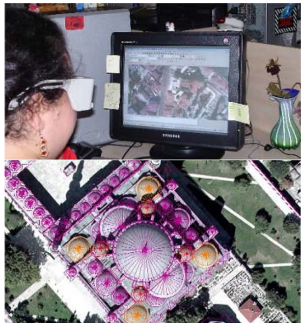
Figure 13. 3D mapping of roofs using Menci-software Z-MAP Foto in stereo mode
