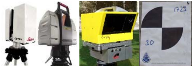
Figure 2. Terrestrial laser scanners used: Leica HDS4500, Leica HDS3000, and Optech ILRIS-3D, target for registration and geo-referencing of scans
