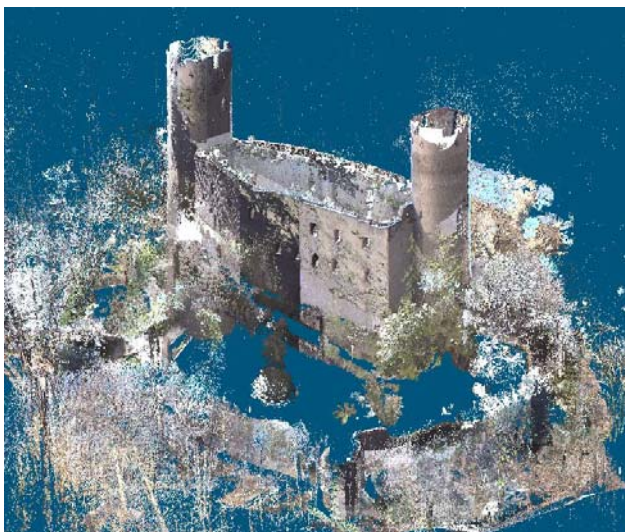
Figure 1. Point cloud currently recorded on the Haut-Andlau Castle
