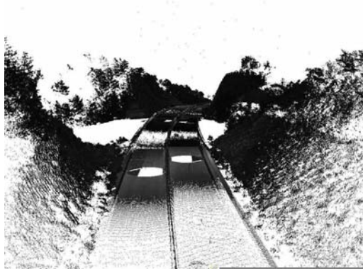
Figure 11. Result of registration from two continuous point clouds measured from each direction
