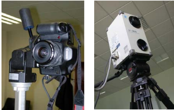
Figure 4. Canon D5 digital camera and 3D laser scanner Minolta VI-900
