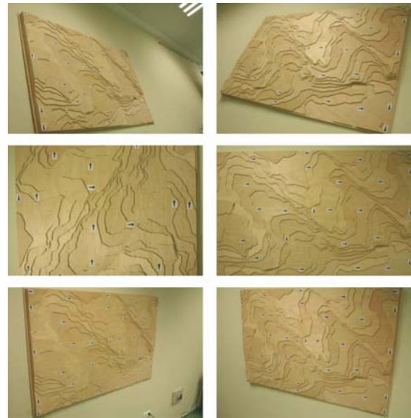
Figure 5. Some photographs of the convergent photo-block for selfcalibration and control/check point network definition.
