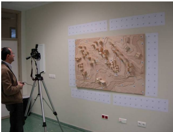
Figure 7. Simulation of photogrammetric flight
