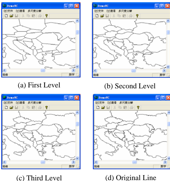
Figure 5 Multi-scale line of four levels
