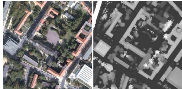
Figure 2. Detail from UltraCamD data set: multispectral and a nDSM
