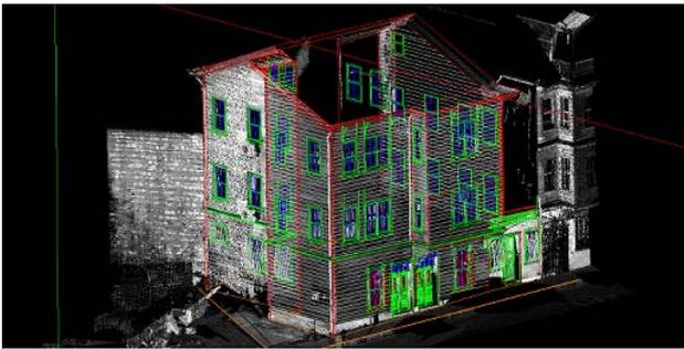
Figure 4. 3D polylines map of building façades based on Z-MAP Laser
