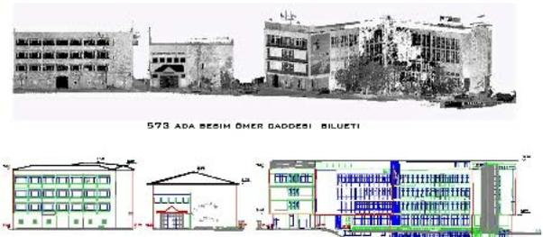
Figure 6. Detailed map of building façades using laser scanning data - laser scanning data (top) and façade plan (bottom)
