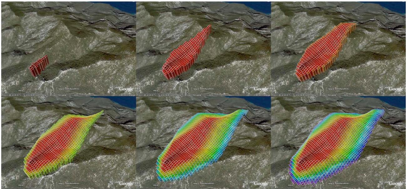
Figure 6: Animation of fire propagation is composed of several frames showing the propagation at different times.
