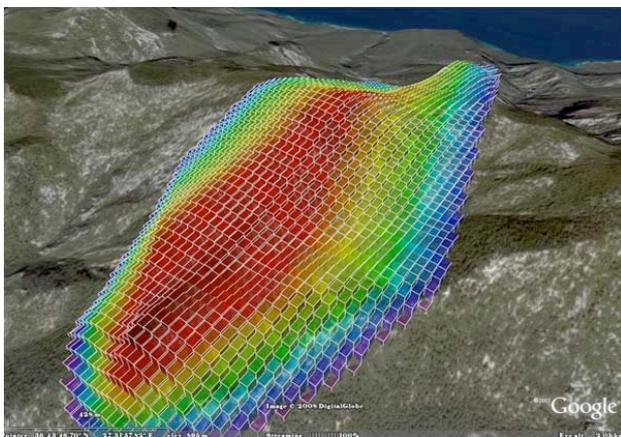
Figure 2: Ignition times using colour coding: red and its tones show the areas which will burn first, while blue and its tones show the areas which will burn later.
