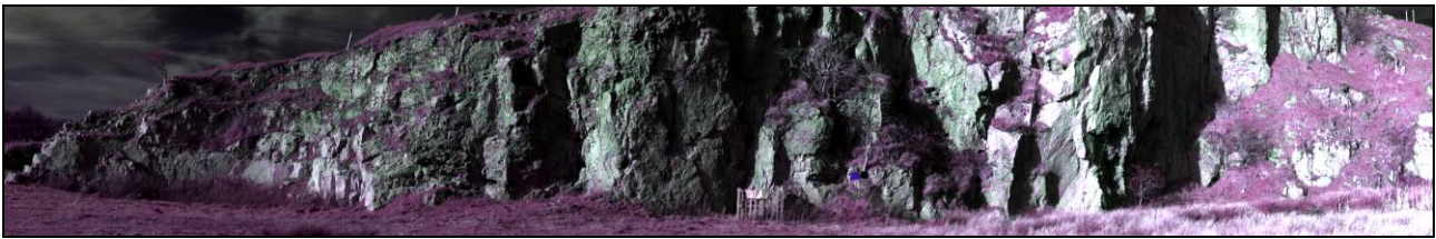
Figure 5. False colour image (Red: 1720 \mu\text{m} , G: 2009 \mu\text{m} , B: 1563 \mu\text{m} ) of Manystones quarry,
