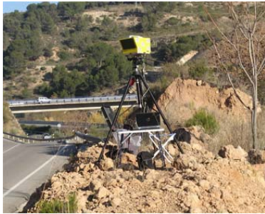
Figure 13. Optech Ilris 3d laser scanner
