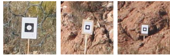
Figure 2. Targets at different distances (approximated). Left: 23 m (the metal net of the barrier is visible behind the target); Centre: 44 m; and Right: 62 m.
