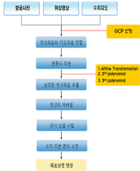
Fig. 5. Flowchart of image processing
